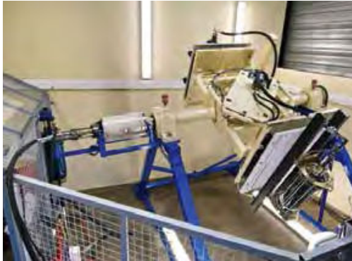
Accumulator test bench for wind turbine application.
