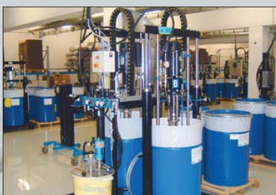
Extrusion pumps 23:1 ratio, used in a multi component skids to transfer silicon
