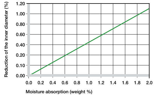
Effect of moisture absorption on iglide® A350 plain bearings
