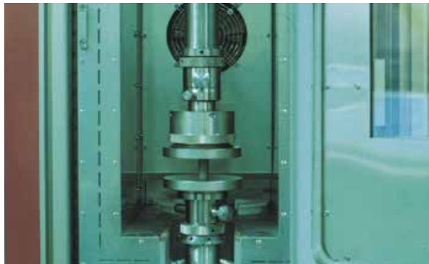
Picture 08: Material tests are possible up to +482 °F
