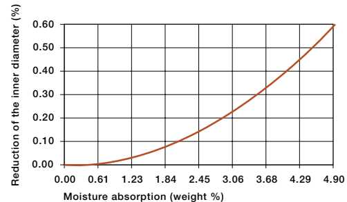
Effect of moisture absorption on iglide® Q plain bearings
