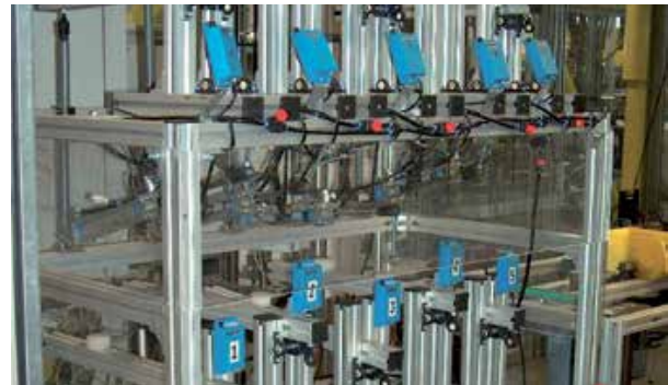
Picture 13: Oscillating wear test rig for testing the wear in oscillating movements at medium loads
