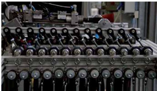
Picture 12: Oscillating wear test rig for testing the wear in oscillating movements at low loads
