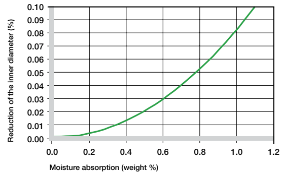
Effect of moisture absorption on iglide® A180 plain bearings
