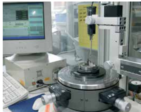
Picture 14: Measurement of the inner diameter of a pressfit plain bearings
