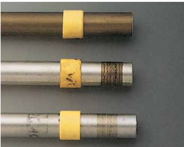
Picture 10: Wear experiments with aluminum shafts
