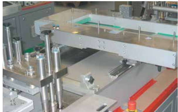
DryLin® W guide rails are accredited to Cleanroom standards and therefore used in this blister machine.
