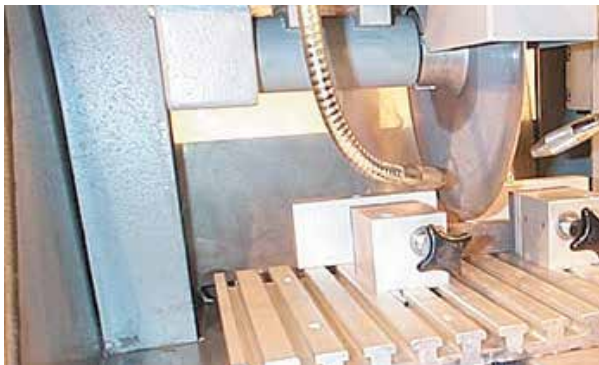
Stainless steel combined with iglide® J in a cut-off grinding machine. DryLin® is resistant to the grinding particles and coolants in the extreme conditions.
