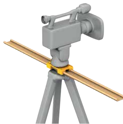
DryLin® W hybrid bearings and W profile guide systems used in camera dollies and sliders.
