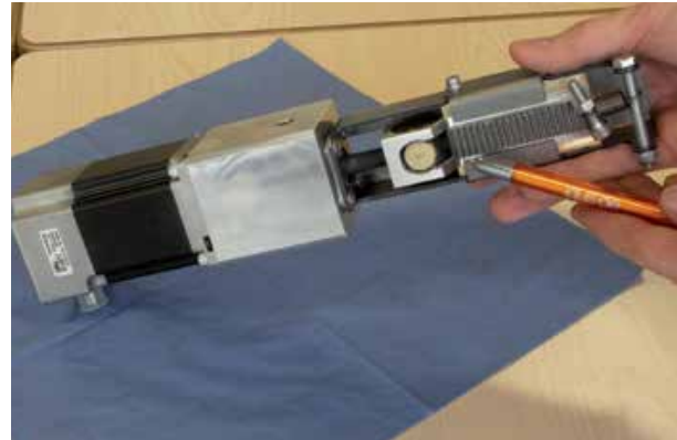
Anti-backlash lead screw nuts in a glue application system of a seam gluing machine (wood industry). These ensure the required precision for this clearance-free adjustment drive.
