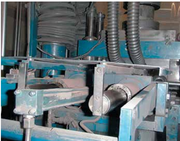
Filling-shoe mechanism in a compaction unit
