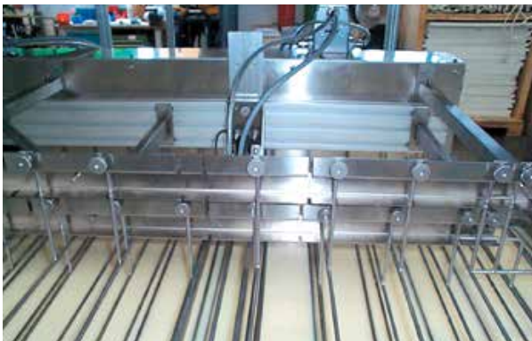
No external lubrication with DryLin® for a baking and conveyor unit
