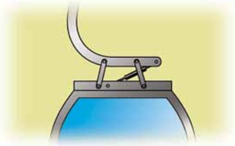
Swinging movements cushioned by hydraulic dampers
