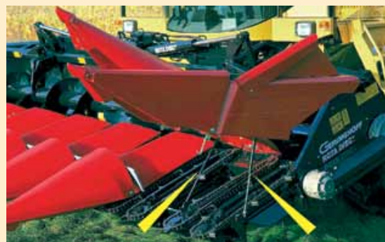
Enhanced protection: Industrial gas springs secure heavy hoods
