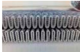
The Filter Media has absorbed water
